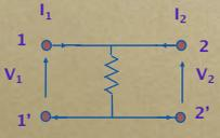
$$G_{12} = \frac{I_1}{V_2} \Big|_{V_1=0}$$
