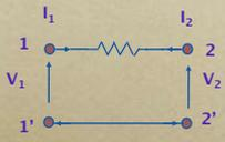
$$R_{12} = \frac{V_1}{I_2} \Big|_{I_1=0}$$
