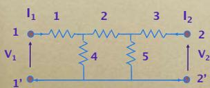
$$R_{11} = \frac{(R_2 + R_5) R_4}{R_2 + R_5 + R_4} + R_1$$
